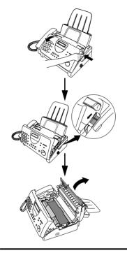
**3** Gently pull the jammed paper out of the machine, making sure no torn pieces of paper remain in the print compartment or rollers.
